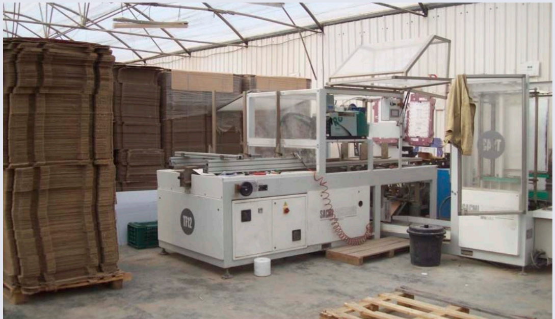
Figure 117. Equipment for the manufacture and printing of the carton paper packages for produce to be exported.
