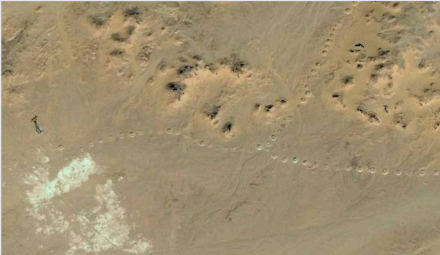
Figure 6. Satellite image of the line of vertical wells of one foggara in the pilot zone.
